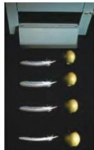
In a vacuum, the apple and feather fall at the same rate and hit the ground at the same time.
